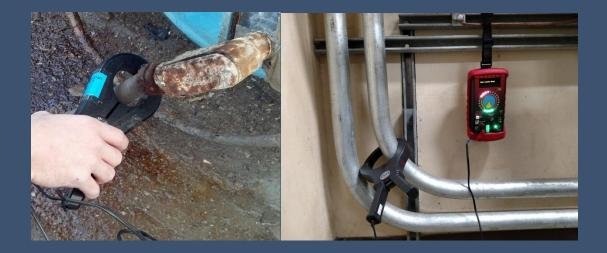
In summary, the ZX3 is an advanced tool by which a DC ground fault can be analyzed for station risk objectives and located without the need to de-energize live vital circuits critical to the station or system. The ZX3 assists in NERC PRC-002-6 compliance, whereby the Station Battery and DC power system must be inspected for inadvertent grounds every four months and aids to overall Nuclear Safety Risk reduction.
