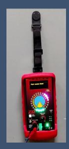
• The Base and Tracer Units have fold out back stands that allow easy viewing when placed on a bench.
