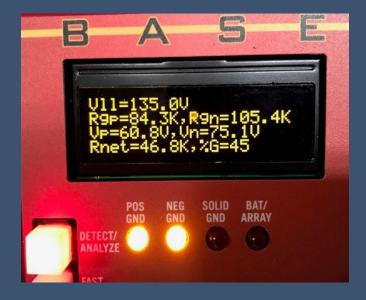
• The ZX3 Base Unit will calculate the "% grounded", thereby allowing the operator to immediately know what potential cell could be cleaned if the source of the ground is at the battery bank or also useful in a multiple ground analysis.
