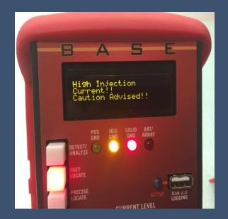
Adjusting the current to below 5.0 mA resets the injection warning level to 6.0 mA.
